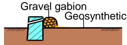
2) Placing geosynthetic & gravel gabions
