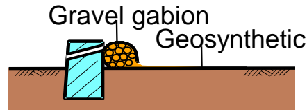
2) Placing geosynthetic & gravel gabions
